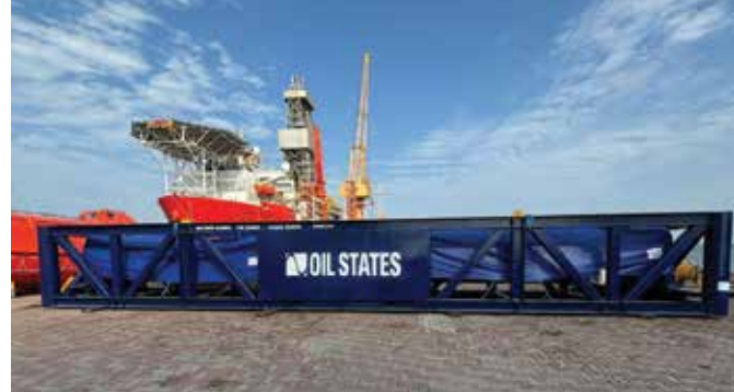
Oil States MPD Integrated Riser Joint loading onto Seadrill's West Polaris rig.
